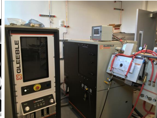
Gleeble 3500 system for thermophysical simulations
