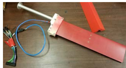
Motion control/damping by piezo actuators mounted on cylinders
